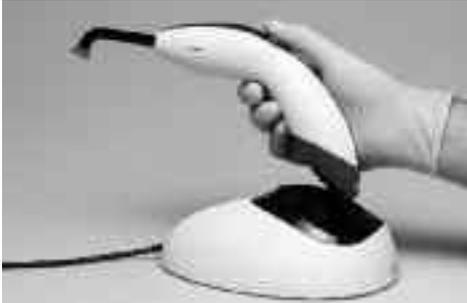
Gently place the handpiece in the corresponding rest in the charging base. If a sleeve is used, please remove it before you charge the battery.
