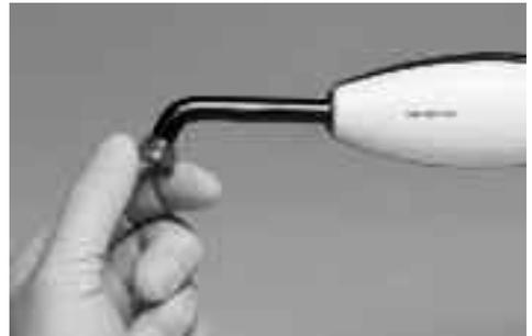
After that, mount anti-glare protection on the light probe.
