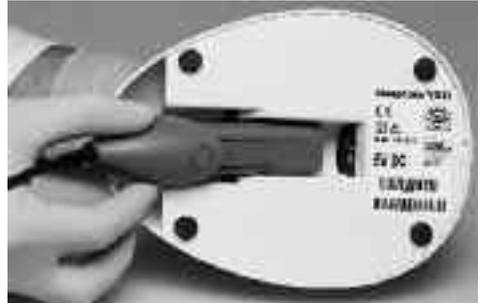
For this purpose, remove the battery from the handpiece. Then remove the power pack from the underside of the charging base. Do not pull on the power cord.
